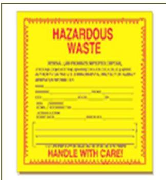
*Hazardous waste containers must be labeled! The label should be filled-out completely, including the facility name and address, type of material, the accumulation start date and generator EPA ID # when ready to ship out for disposal.*
